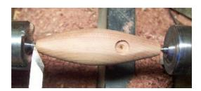
If you purchase the Wooden Lure Blocks and plan to drill eyes holes for the 3D molded eyes; I suggest the use of a forstner bit for this job. Forstner bits and 3D molded eyes are available in various sizes. Details on how to build a lure block holder for drilling eye holes are available in the e-book on Lure Making at <a href="http://www.woodenluremaking.com">http://www.woodenluremaking.com</a>
