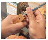
When turning the lure blocks on a lathe; turn the lure blocks all the way to end of the block. In other words; the lure block length you begin with should be the length of the finished lure. Doing it this way ensures the holes for the eye screws are in the dead center on the ends of the lure and that each additional lure of this type is exactly the same length.
